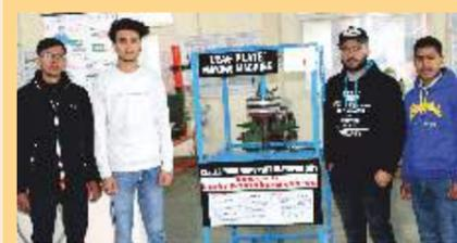
**Pattal Making Machine:** There is an ample opportunity for the traditional patravali due to its environment-friendly nature and biodegradability. An attempt of fabricating low-cost and more ergonomic pattal making machine is hereby made. The machine is manually operated by a foot pedal, has a fixed upper die and a moveable lower die, and is composed of a heating element.
